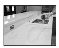
AFTER MIXING THE COMPONENTS, YOU HAVE ABOUT 30 MINUTES TO COMPLETELY COAT THE SECTION before it stops flowing adequately. It takes about 5 to 10 minutes to coat one 6-foot section.
