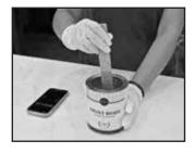
Then, using a stir stick, stir the epoxy mixture vigorously for **3 minutes and 30 seconds**. You **MUST** scrape the sides and bottom to mix thoroughly. Failure to do so will result in improperly mixed epoxy that will not cure correctly.
