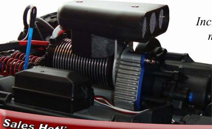
Includes, Blower assembly, air scoop, mounting bracket and drive belt.
