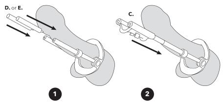
Your product arrives with four threaded extension rods for a customizable length. Simply screw the desired extension rods end to end to attach. Then, bend the base down for use.
