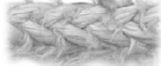
Rope must be replaced
