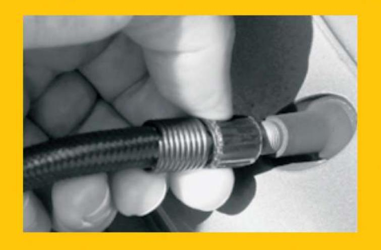
Screw connector on air valve stem
