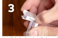
Install the latch on installation tool
