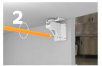
Mark the lock's 4 pilot holes with a
