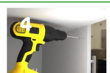
Put away the lock and latch, and get a wood drill bit with a 0.5mm (1/32") diameter.
