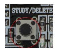
④ Press any key on the control panel to learn from the control board. Then you can remote control the gate motor by your smart phone now.
