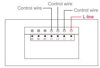
Connect the wires as shown above, tighten the screws and check for firmness.
