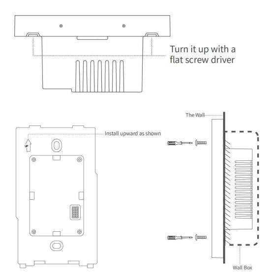
Depth of the wall box should be more than 50mm.
