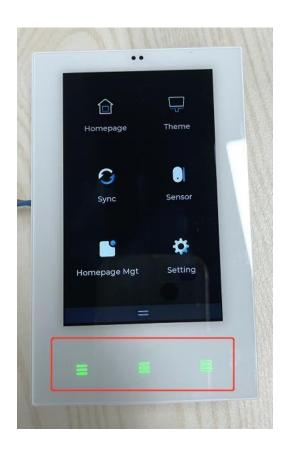
Long press switch 1 or switch 2 or switch 3 to change the name of the switch.
