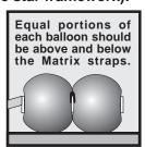
(B) To load balloon in double layer (Use two star frameworks): Size balloons without squeezing them first.
