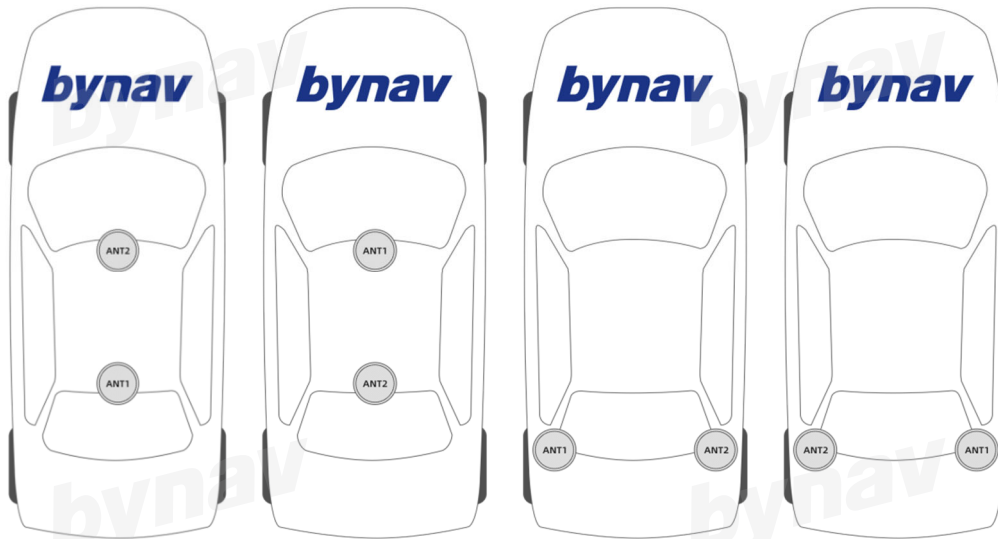
Figure 14 Antenna Installation Method
