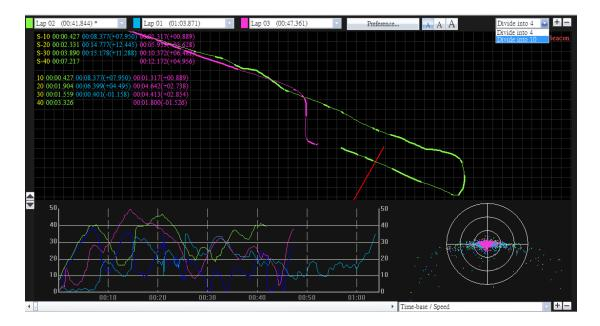
In Map View, you can give tags on the track or on the graph line with three different colors, red, green, and white. You can mark the position for define accelerate point or break point purpose.
