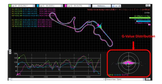
Show Brake line: It can show you the braking line on the track. You can compare the tracks and get acceleration and braking information. (The thick lines present the braking zone, and the thinner lines present the acceleration zone.)
