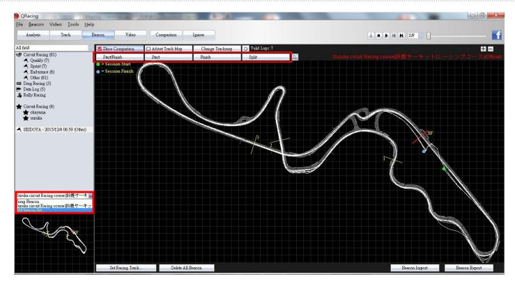
You can click on refresh lap button to re-calculate the Valid lap numbers, for example you adjust the start/finish line or Split line position.
