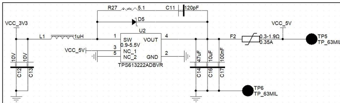
**Figure3-2 5V boost circuit**
