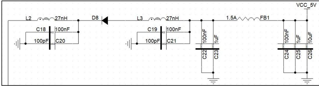
**Figure3-9 Antenna Feeding Circuit**
