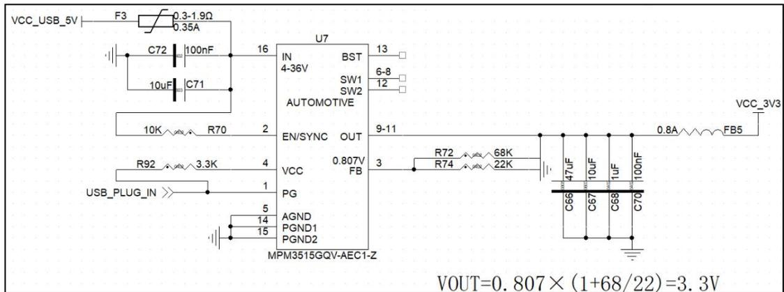
**Figure3-3 3.3V step-down circuit**
