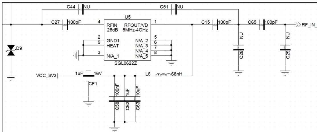
**Figure3-10 low-noise amplification circuit**
