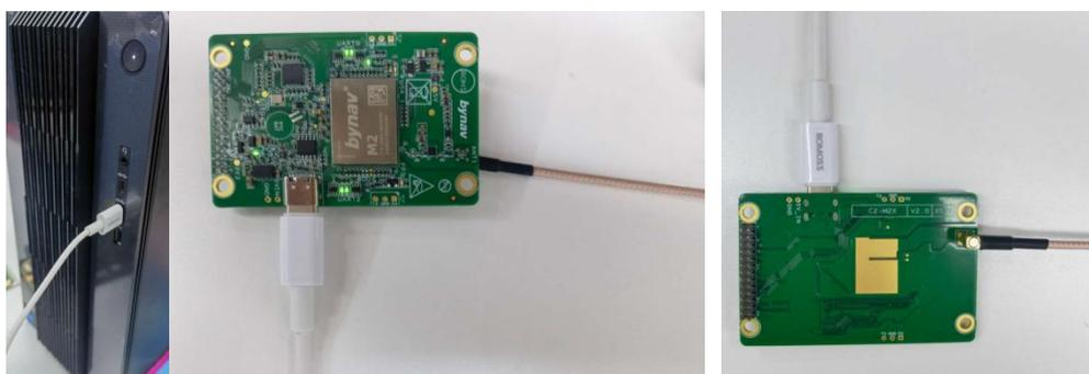
Figure4-2 Device connection
