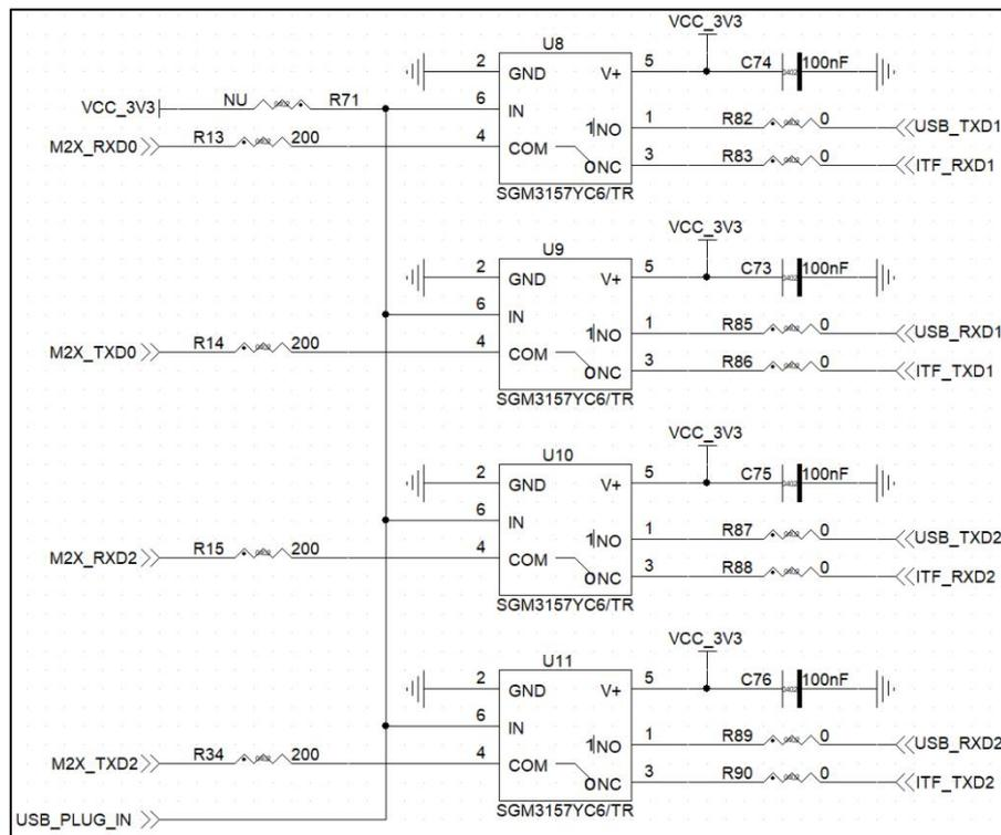
**Figure3-6 analog switch circuit**
