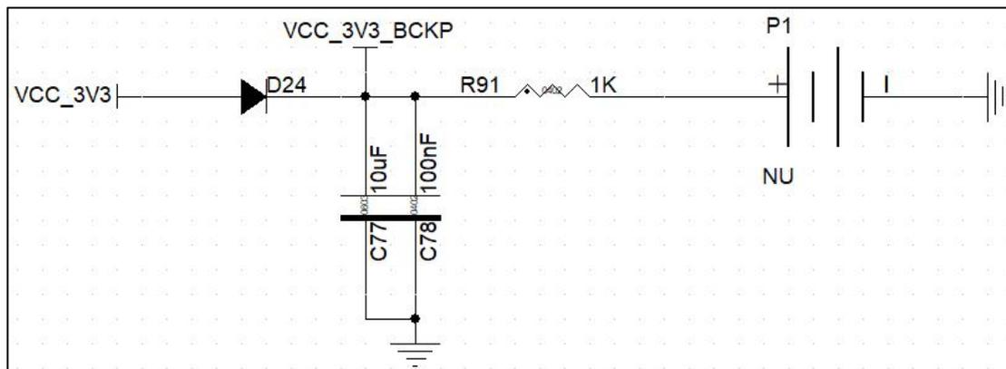
**Figure3-4 RTC circuit**
