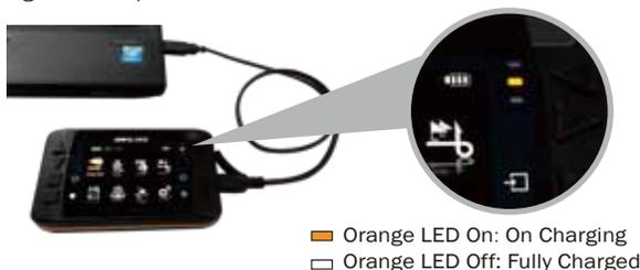
※ Charging time is typically 5 hours when device power is Off.
