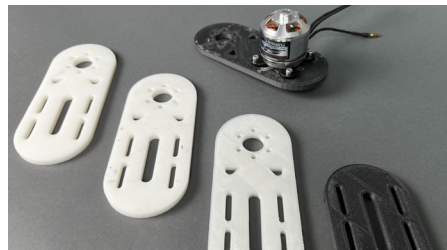
Test iterations laid out with Final print & motor installed
