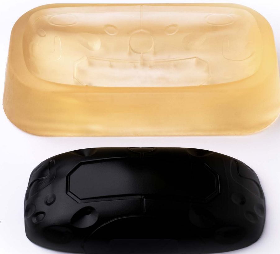
Multiplier-made product casing prototype and 3D printed template
