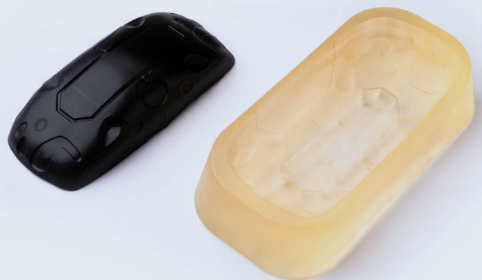
Multiplier-made product casing prototype and 3D printed template
