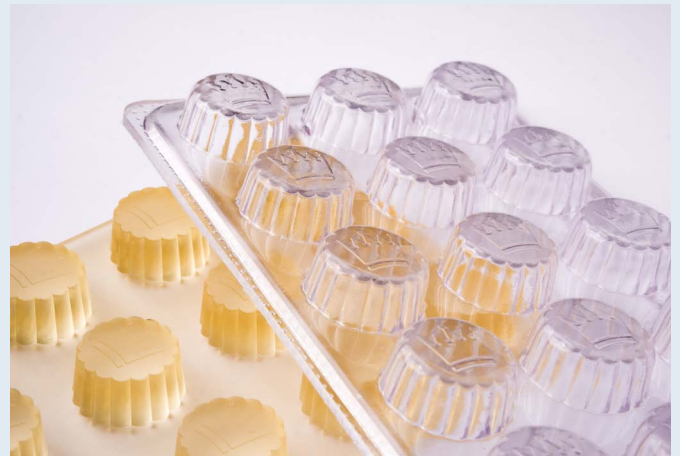
Multiplier-made food mold prototype and 3D printed template
