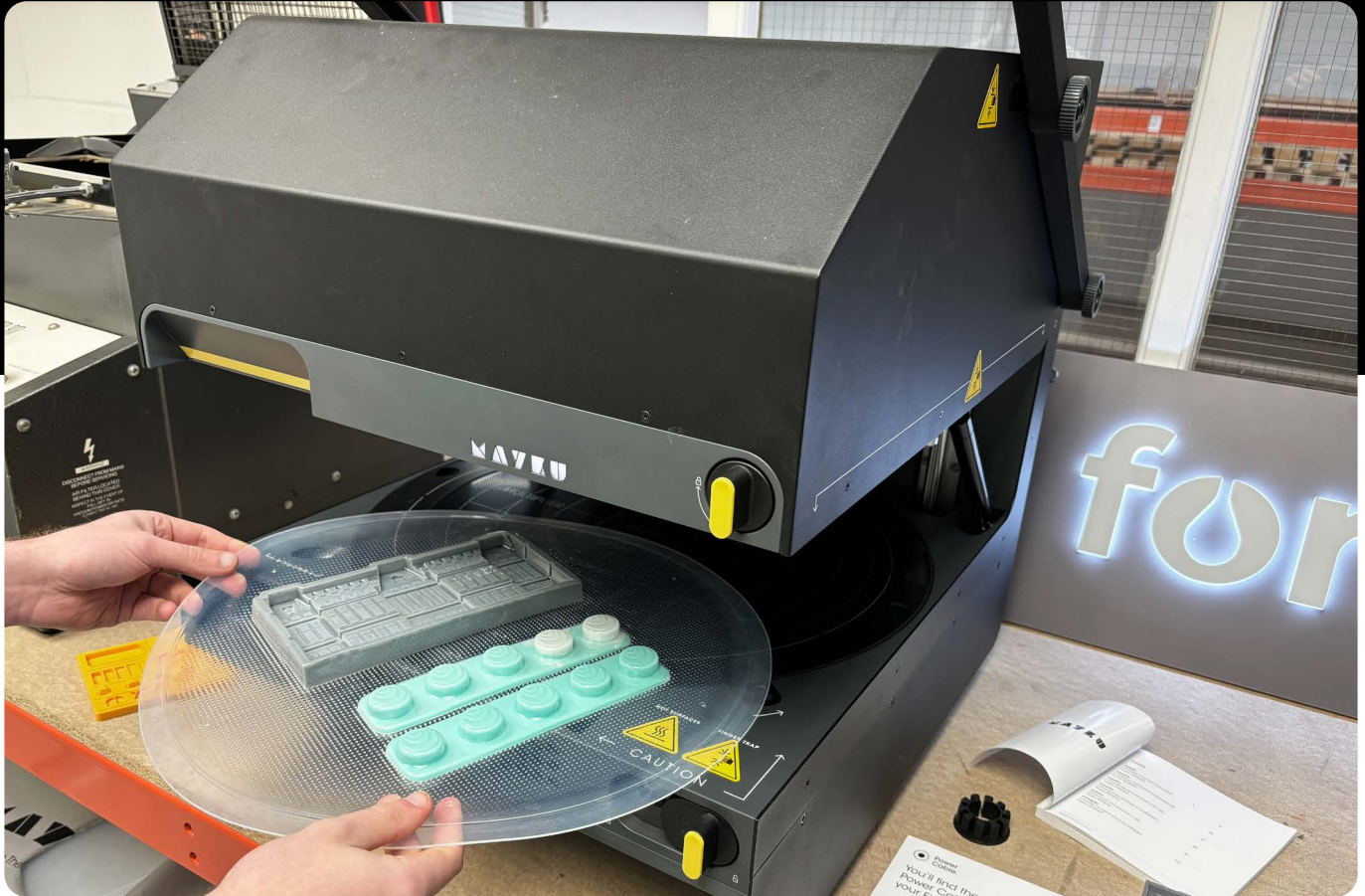
Above: Form being removed from the Mayku Multiplier
