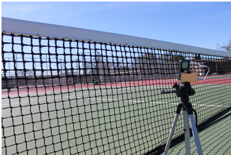
Radar behind the net, mounted to tripod and powered via USB Power Pack
