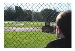
3. Attach the radar (attached to the Universal Mount) to the chainlink fence behind the backstop in-line with the pitcher. You can use your mobile device to remote control the radar, by pressing "Start" inside the app on the video screen. That's really the power of the app, it allows you to capture accurate speeds with the radar while being able to set up off to the side, etc. You can also zoom in on the pitcher inside the app.
