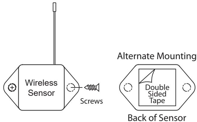
In order for your wireless sensors to work optimally, you should orient all antennas for your sensors and gateway(s) the same direction (typically vertical). Also sensors must be at least 3 ft. away from other sensors and the wireless gateway in order to function properly.
