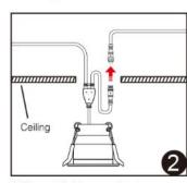
Connect lights according to connection diagram.
