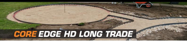
The CORE Edge HD Trade range is manufactured from 2.5mm mild steel and is hardy enough to handle vehicular traffic. The 2275mm edgings are ideal for larger applications as it cuts down the number of connections and reduces the install time. They can easily form both straight lines and curved radius, or be bent on site to form precise angles. It provides the perfect edge restraint in a variety of landscaping applications.
