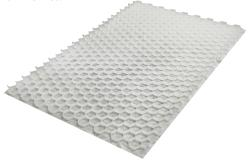
Both the large sheet (2400x1200mm) and the small sheet (1200x800mm) come with an 80gsm non-woven weed membrane heat welded to the underside of the grid. This not only prevents weed growth from beneath the surface, but also prevents the gravel from migrating under the cell wall and into the sub base over time.
