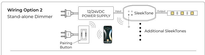
If you are installing more than one Wall Switch unit, all others must be switched Off while pairing.
