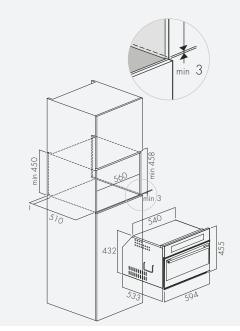
AO450X Series Oven Specifications Total Electrical Consumption: 2.6 kW/H Electrical Connection: 15AMP GPO/Hard connection
