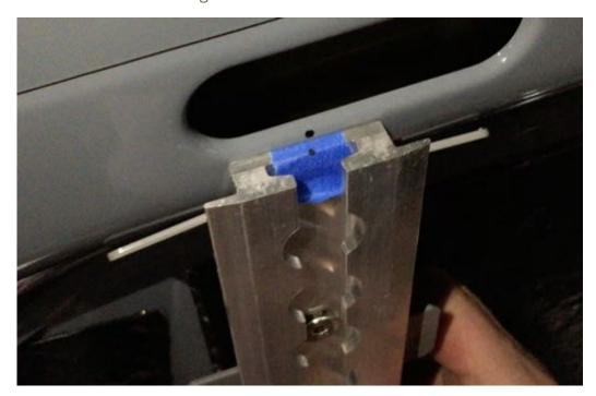
The L Track that is mounted to the bracer should sit flush with the side of the van. It is ok to have 1-2mm spacing, but flush is preferred as this will mate up with the rest of the Adventure Wagon RUV interior kit.
