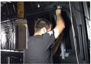
Typically the top of the bracer "ears" prevent it from seating into the slightly curved frame of the van. Use a rubber mallet and tap/bang the end of the bracer ears on both side to allow for a tighter fit.
