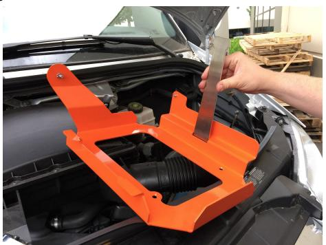
6. Place the tray tray into the driver side engine compartment. Align tab (A) with the hole in the firewall, Tab B will slot into the available hole in the wheel well housing. The holes in area (C) will align with the existing battery mount holes at the base of the tray
