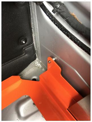
9. Attachment (C) to the engine compartment frame. Attach two stainless M6 bolts on the topside fastened via a washer and nylon locking nut from the bottom side.
