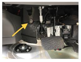
8. Attachment (B) to the engine compartment sidewall. The stainless post should be placed into the opening on the side of the van. No additional fastening is needed
