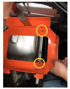
10. Place two group GC2 6 volt batteries in the tray and assemble side bolt down bracket and top hold down per the photo below with stainless nuts.
