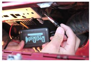
Insert the RediRad's male cable into the radio's antenna jack.
