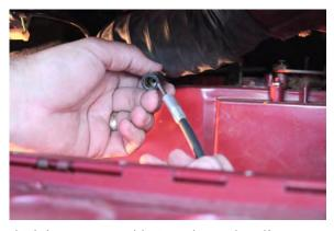
Insert the vehicle's antenna cable into the RediRad's antenna jack.
