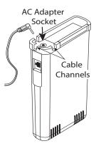
Note: WeatherLink Live is powered by AC power with battery backup. **AC power is** required; it cannot be set up or run on batteries alone. Since WeatherLink Live does not store data, it is highly recommended that you install batteries to prevent loss of data if AC power is lost.
