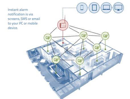
The above schematic shows an example of RF500 mesh network. In the event of signals being blocked to or from a specific route, RF500 Transmitters automatically seek an alternative route across the mesh network.
