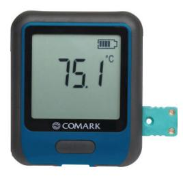
temperature via a range of Comark thermocouple probes. The probe can be used in a wide range of temperature situations such as measuring core food temperatures during cooking and in hot holding cabinets or wells.
