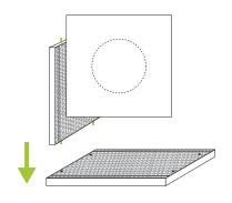
Align a Side zBoard to Bottom zBoard and Entry zBoard as shown.
