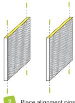
Place alignment pins in vertical zBoards.
