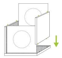
Align other Side zBoard to Bottom zBoard and Entry zBoard as shown.
