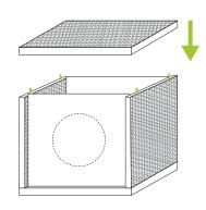
Align Top zBoard to unit and press down firmly to secure.
