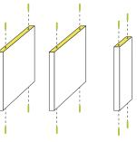
Insert alignment pins to side zBoards and middle zBoard.
