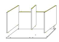
Align vertical zBoards to horizontal zBoard as shown. Press down firmly.
