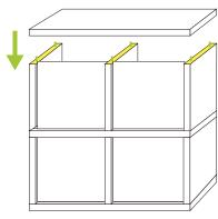
Align top horizontal zBoard to unit and press down firmly.
