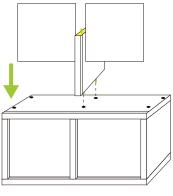
Align vertical middle zBoard to horizontal zBoard and press down firmly. Insert backboards into grooves.
