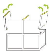
Align vertical side zBoards with grooves facing the backboard.
