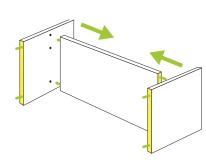
Carefully remove the protective layer leaving the 3M adhesive on zBoard (adhesive shown in yellow).
