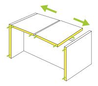
With adhesive on zBoard all facing same direction, align left and right Backboard to side zBoards.
