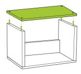
Next, align middle horizontal zBoard (there will be holes on both sides of board) on top of vertical zBoards.
