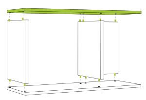
Start with the bottom horizontal zBoard (there will be holes on only one side of board).
