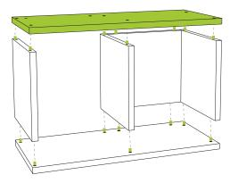
Start with the bottom horizontal zBoard (there will be holes on only one side of board). Align vertical zBoards to holes in the horizontal zBoard.
