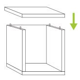
Align horizontal zBoard and press firmly to secure unit together. Visit links below for more details.
