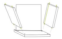
Arrange vertical zBoard with grooves facing backboard as shown.
