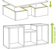
Align Back zBoard and press firmly to secure unit together. Flip right side up as shown.
