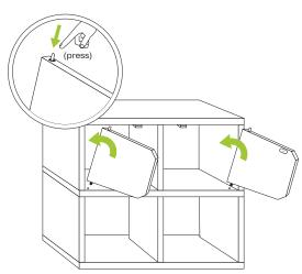
Position doors as shown. Align bottom door pin to hole. Press on spring loaded top pin and insert.
