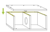
Align Top zBoard (with door stopper) as shown and press firmly to secure unit together.
