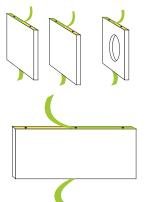
Carefully remove the protective layer on the Side zBoards, Middle zBoard and Back zBoard (making sure not to remove the 3M adhesive). Tip: Peel protective layer from
