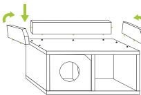
Align Short Back zBoard and Short Front zBoard to holes in Top zBoard.
