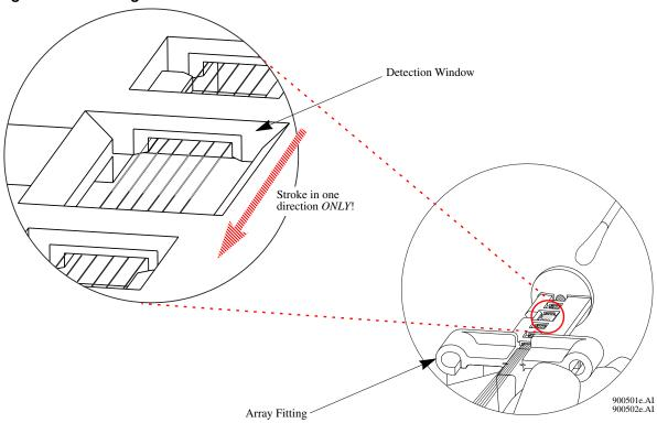
Figure 218: Cleaning the Detection Window
