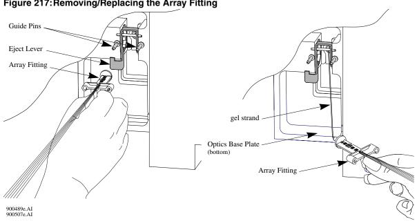
Figure 217: Removing/Replacing the Array Fitting
