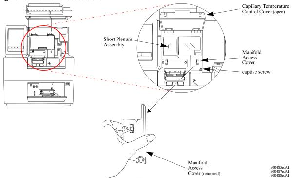
Figure 201: Manifold Access Cover
