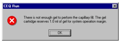
You will also be presented with the dialog box in Figure 87 if you attempt to run a sample plate and the gel cartridge does not have enough gel to process any sample sets in that plate.
