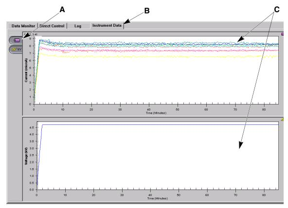
Figure 36: Run Module, Instrument Data Window
