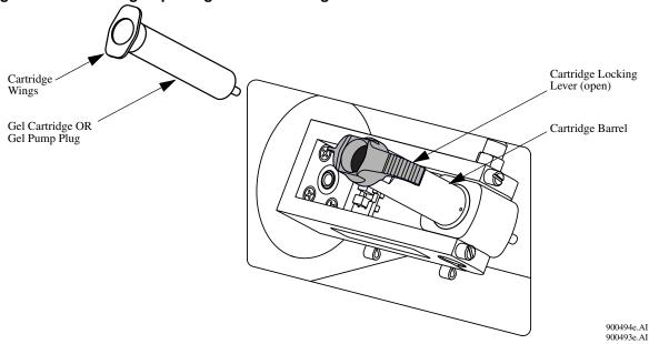
Figure 209: Removing/Replacing the Gel Cartridge - Continued
