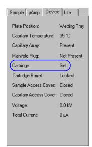
Figure 89: Device Tab – Gel Plug installed
