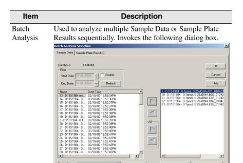
Once files are transferred to the right-side list box and **OK** is selected, the analysis parameters editor dialog box is displayed. Select the appropriate analysis parameters or edit an existing parameter set and click **OK**, batch processing begins and a window, similar to the one below, is displayed.
