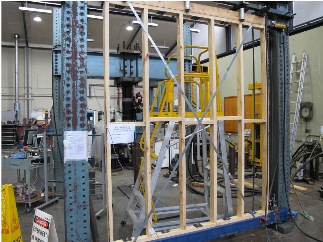
Figure A1 Test set-up for the 450mm studs wall
