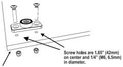
Place on a flat surface and fasten with included machine screws and nuts. (Up to 15mm thickness).
