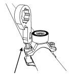
Use a 9.Solutions GoPro Multi-tool or a 3/16" allen key to fasten mount to a pole, handle bar, or roll bar.
