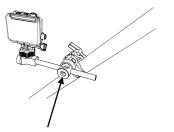
The unit can used in combination with a any 3/8" (10mm) or 3/8" female threaded equipment.
