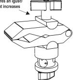
Replace the discs on a grip head with the Python Clamp to allow a wider a range of clamping possibilities on flat objects, large tubes, or any odd shaped object.
