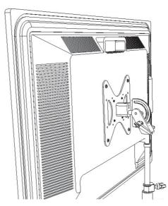
The large VESA to 5/8" Receptacle can be usedwith any 5/8" pin fitted equipment like the Tilt adaptor.
